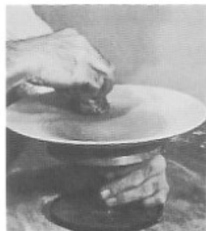
Sponge Spinning: Round shape turned on banding wheel; sponge feeds color.
